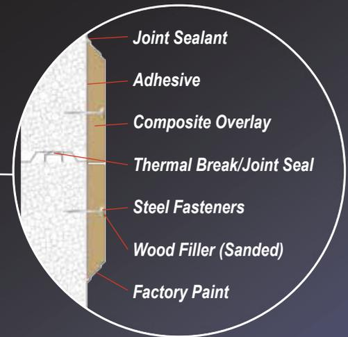
Door panel design segments are precision computer cut from a single sheet of wood composite overlay material.
